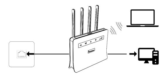
**Scenario 3:** Data service from Ethernet cord and VOLTE voice using a SIM card
