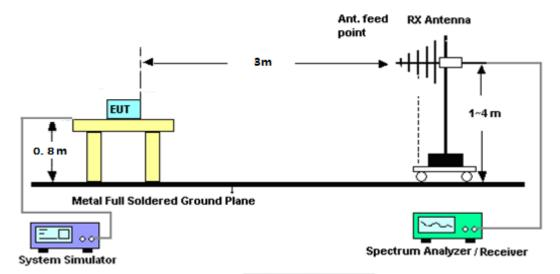
For radiated test from above 1GHz
