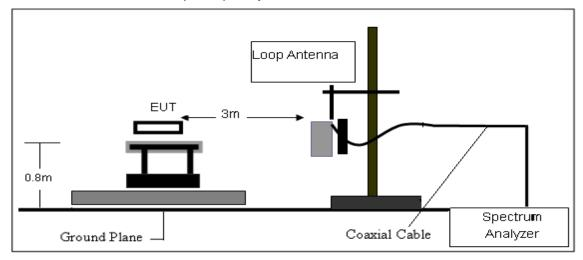
(B) Radiated Emission Test-Up Frequency 30MHz~1GHz
