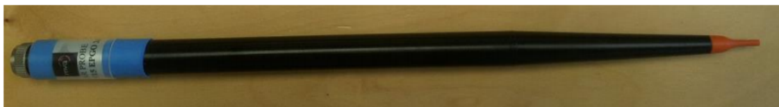
Figure 1 – MVG COMOSAR Dosimetric E field Dipole
