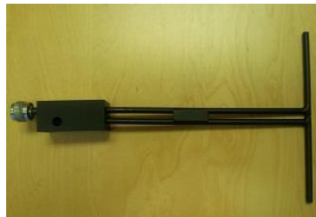
Figure 1 – MVG COMOSAR Validation Dipole
