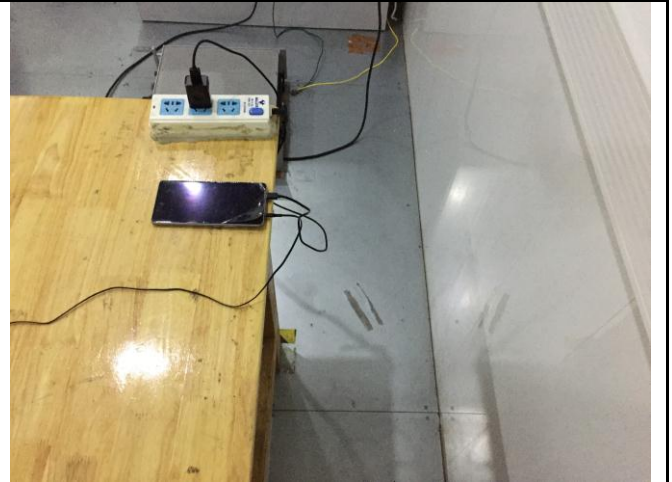
Conducted Emissions Test Setup Side View
