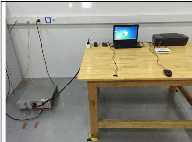
Conducted Emissions Test Setup – Front View
