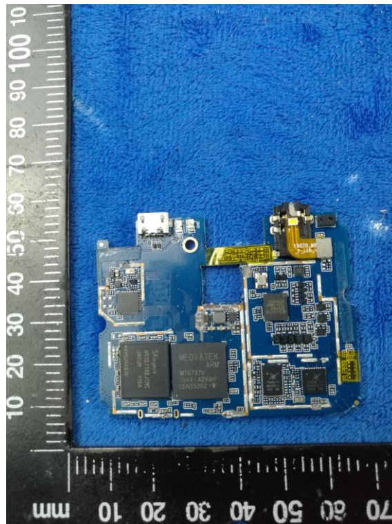
Mainboard without Shielding – Rear View
