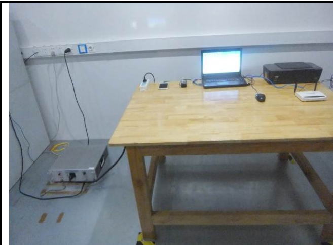
Conducted Emissions Test Setup – Front View
