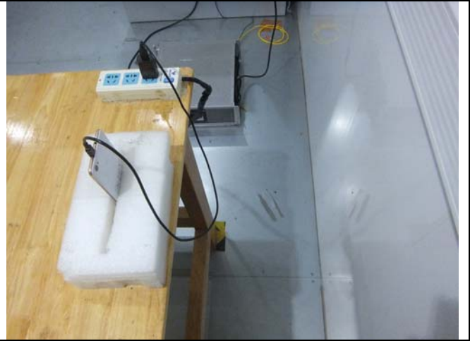
Conducted Emissions Test Setup Side View
