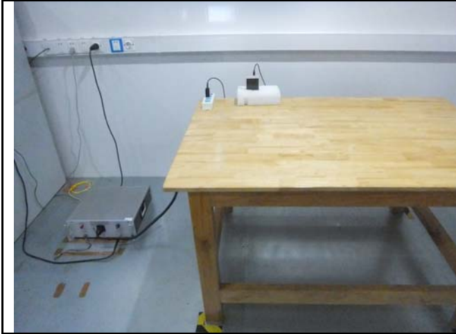
Conducted Emissions Test Setup Front View
