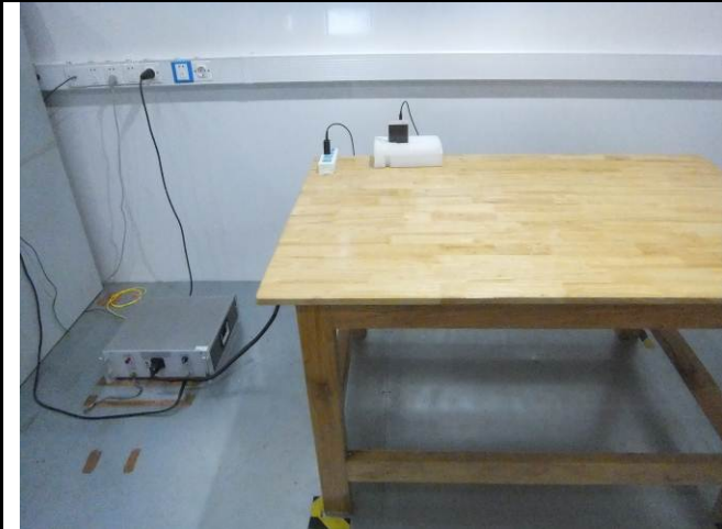
Conducted Emissions Test Setup Front View
