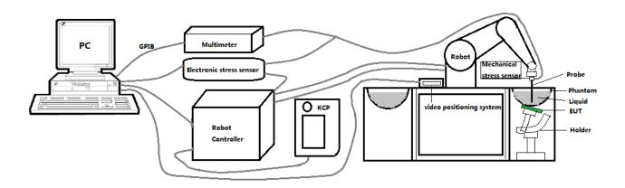
These measurements were performed with the automated near-field scanning system OPENSAR from SATIMO. The system is based on a high precision robot (working range: 901 mm), which positions the probes with a positional repeatability of better than ±0.03 mm. The SAR measurements were conducted with dosimetric probe (manufactured by SATIMO), designed in the classical triangular configuration and optimized for dosimetric evaluation.
