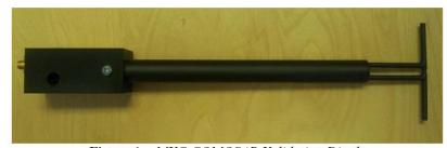
Figure 1 – MVG COMOSAR Validation Dipole
