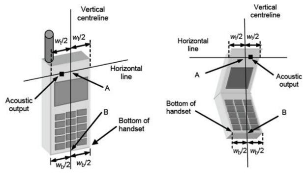
Fig 6.2.1 Handset vertical and horizontal reference lines—"fixed case
