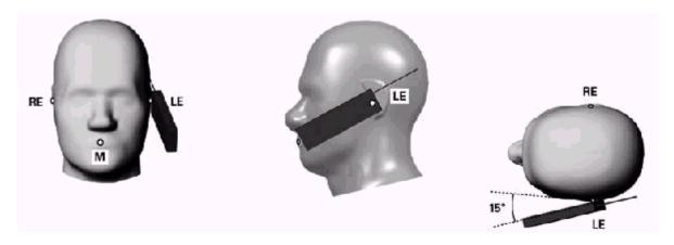
Figure 6.3.1 – Tilt position of the wireless device on the left side of SAM
