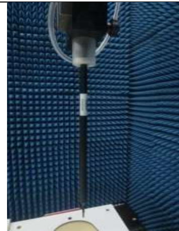
Fig.8.2 Photo of E-Field Probe
