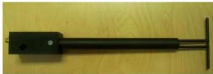
Figure 1 – MVG COMOSAR Validation Dipole
