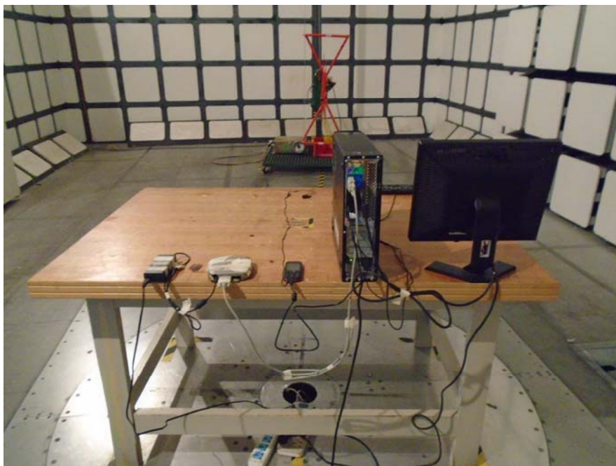
Radiated Emissions – Rear View (Below 1 GHz)
