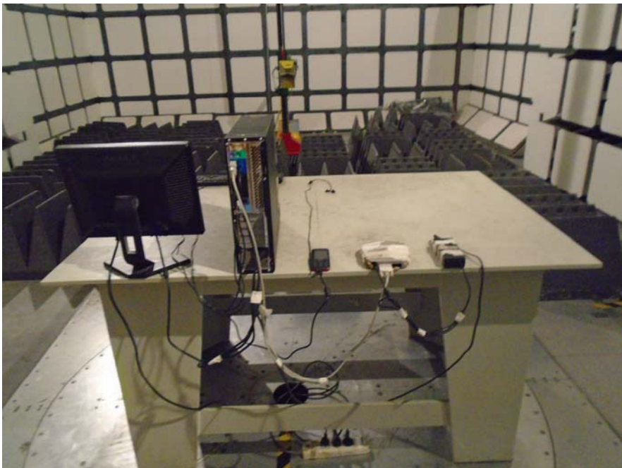
Radiated Emissions – Rear View (Above 1 GHz)
