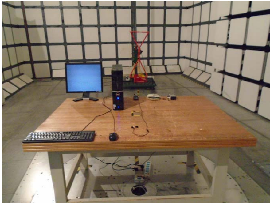
Radiated Emissions – Front View (Below 1 GHz)
