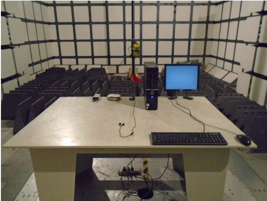
Radiated Emissions – Front View (Above 1 GHz)
