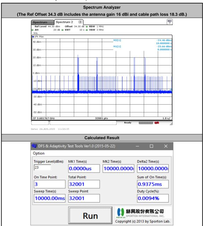
The sum of On Time (aggregated time from marker 1 to 2): 0.93ms < 1s, Pass.
