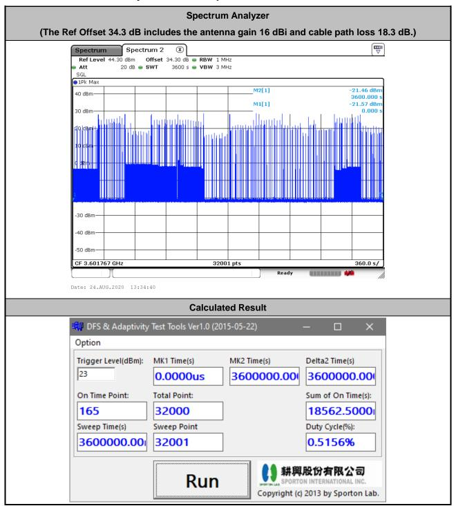
The sum of On Time (aggregated time from marker 1 to 2): 18.56s < 20s, Pass.
