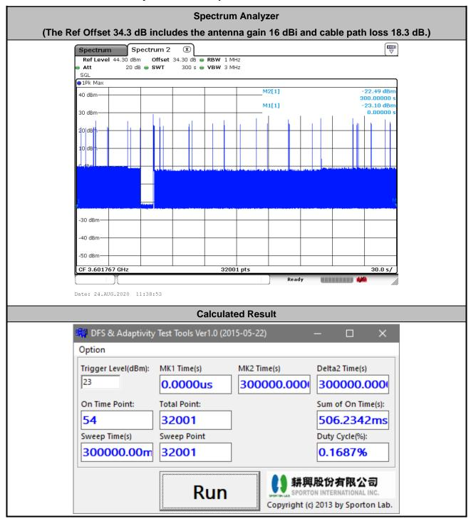
The sum of On Time (aggregated time from marker 1 to 2): 506.23ms < 10s, Pass.
