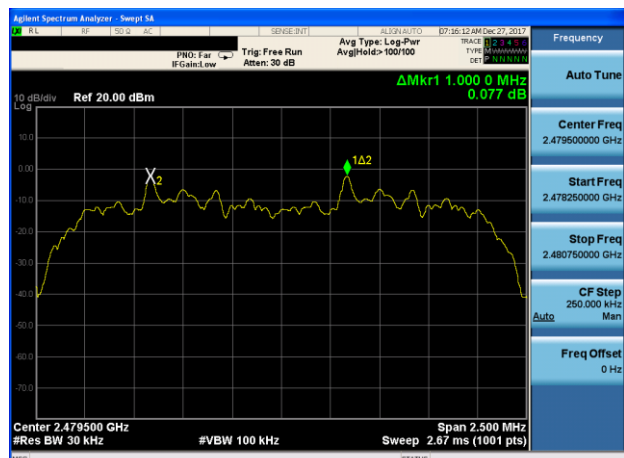
(2Mbps) Channel Separation plot on channel 77-78
