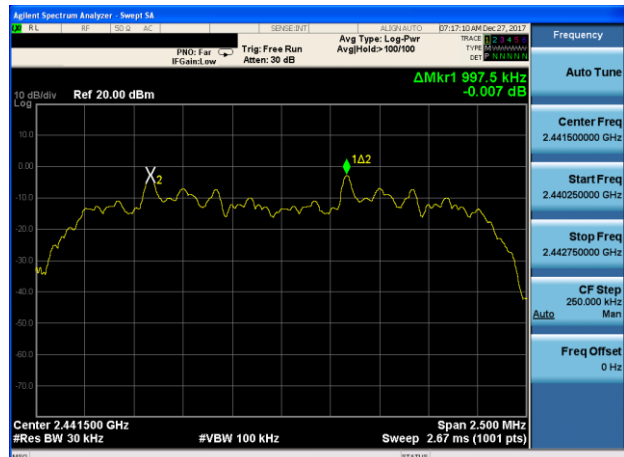
(2Mbps) Channel Separation plot on channel 39-40
