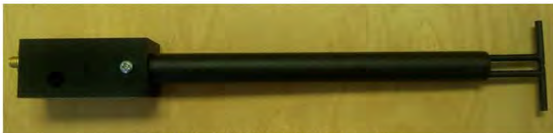
Figure 1 – MVG COMOSAR Validation Dipole
