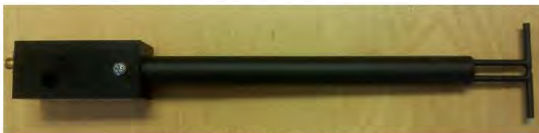
Figure 1 – MVG COMOSAR Validation Dipole
