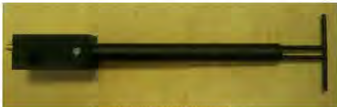
Figure 1 – MVG COMOSAR Validation Dipole
