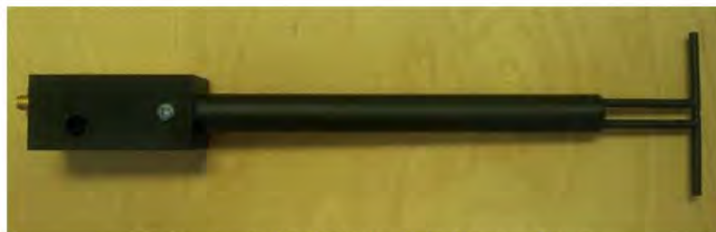
Figure 1 – MVG COMOSAR Validation Dipole
