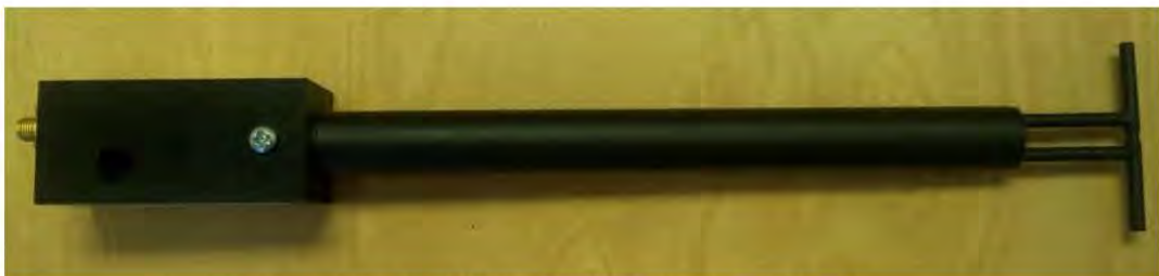
Figure 1 – MVG COMOSAR Validation Dipole
