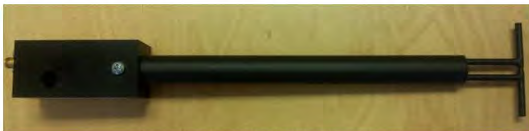
Figure 1 – MVG COMOSAR Validation Dipole
