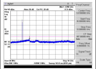
Conducted Emission Transmitting Mode CH 4233 5GHz – 10GHz
