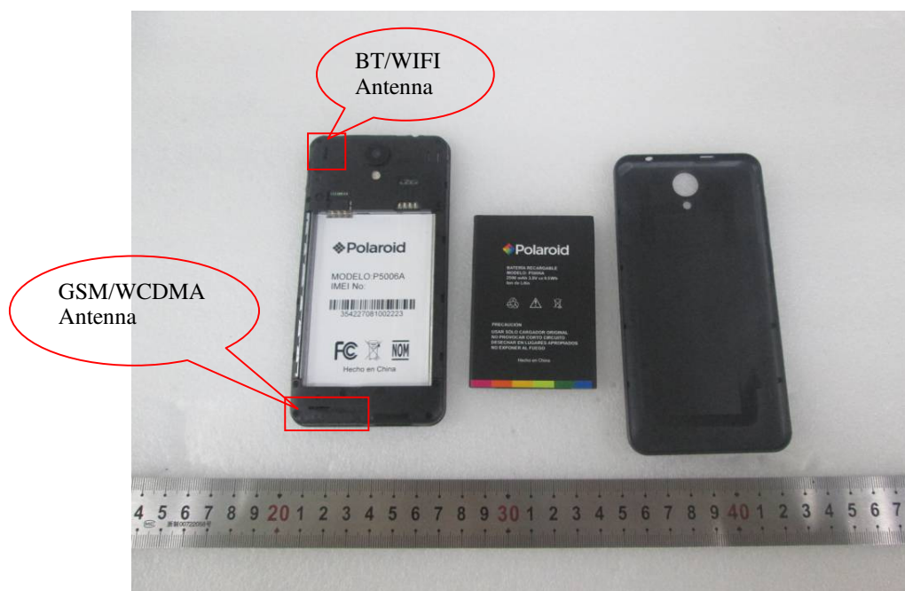
EUT – Cover off View 2
