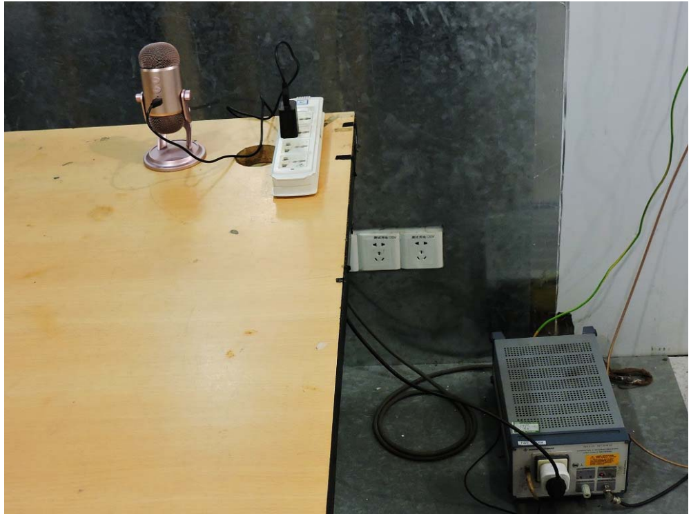
Conducted Emission Test Setup:
