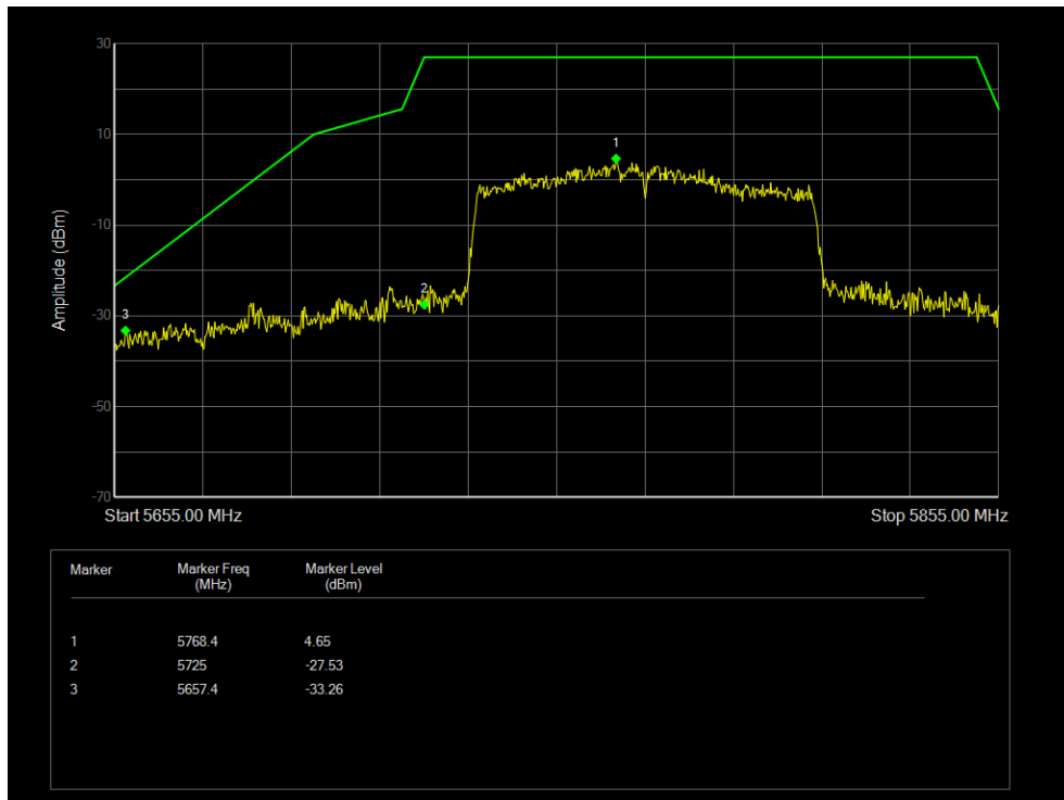
Band Edge NVNT 802.11n(HT20) 5745MHz Low Ant1
