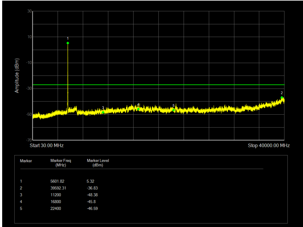
Tx. Spurious NVNT 802.11ac20 5700MHz Ant1 Emission
