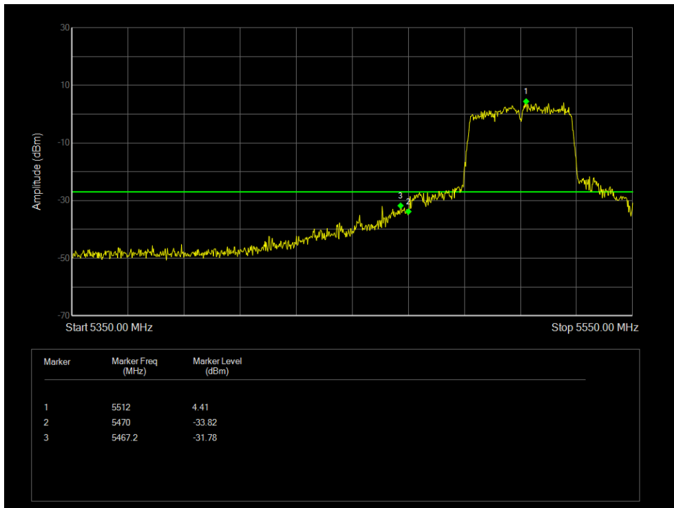
Band Edge NVNT 802.11ac40 5670MHz High Ant1
