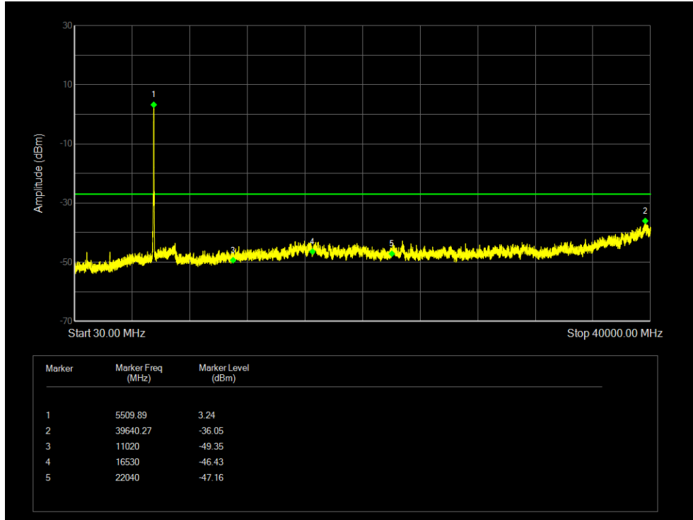
Tx. Spurious NVNT 802.11ac40 5590MHz Ant1 Emission
