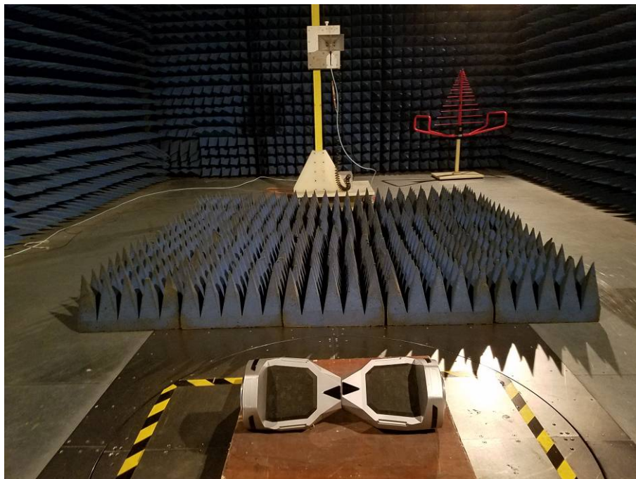
RADIATED EMISSION TEST SETUP (ABOVE 1 GHz) FROM 0.1M-HEIGHT TEST TABLE
