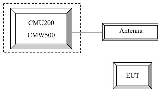
**Block Diagram of Test Setup**
