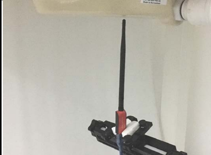
Test Position 5: USB Tip with 0.5 cm Gap(Antenna 0 degree)
