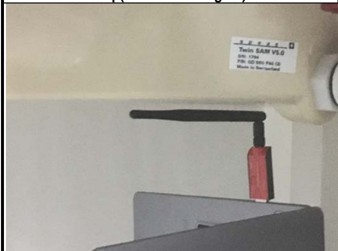
Test Position 15: USB Tip with 0.5 cm Gap (Antenna 90 degree)
