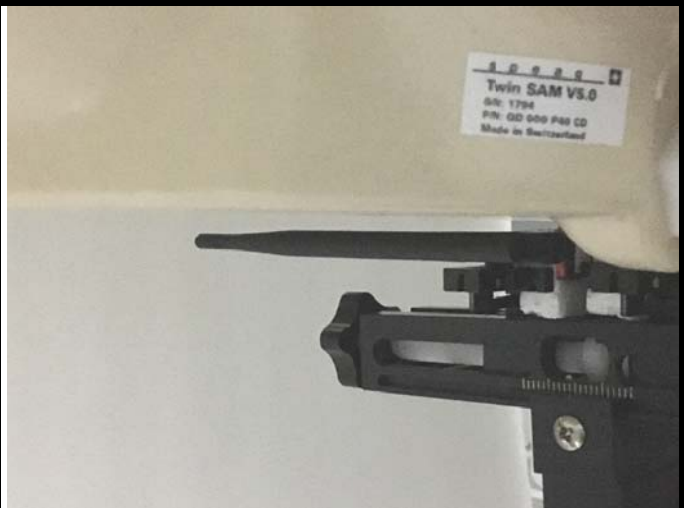
Test Position 14: USB Vertical Back With 0.5 cm Gap (Antenna 90 degree)
