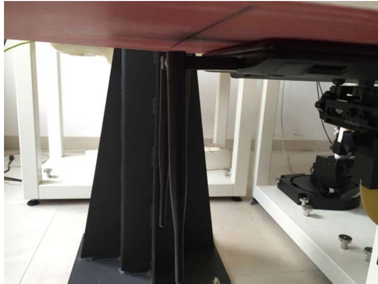
Test Position 1: 5 mm separation from the flat phantom for the bottom of the dongle at Horizontal-Up;
