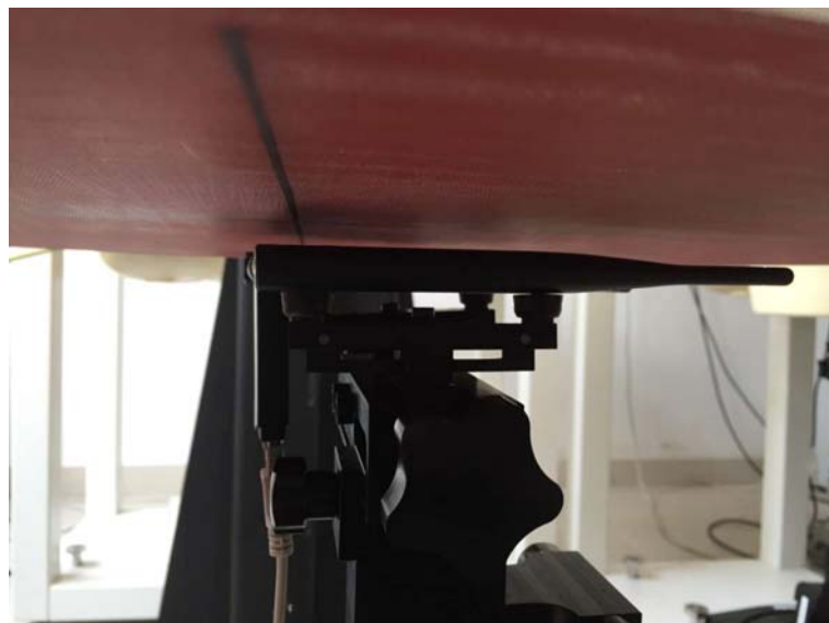
Test Position 3: 10 mm separation from the flat phantom for the end of the dongle (opposite from the USB connector);
