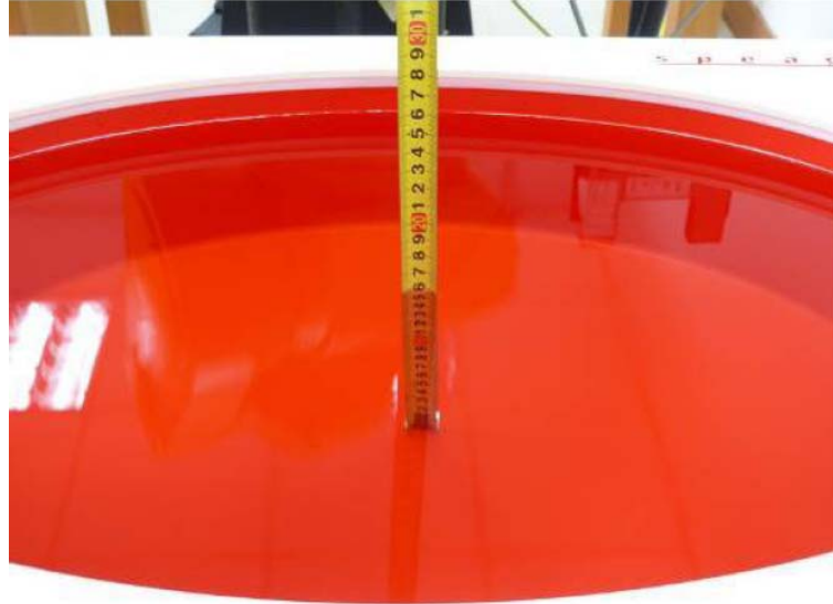
Photograph of the depth in the Body Phantom (2450MHz, 15.4cm depth)
