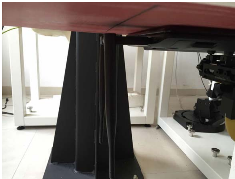
Test Position 1: 5 mm separation from the flat phantom for the bottom of the dangle at Horizontal-Up;
