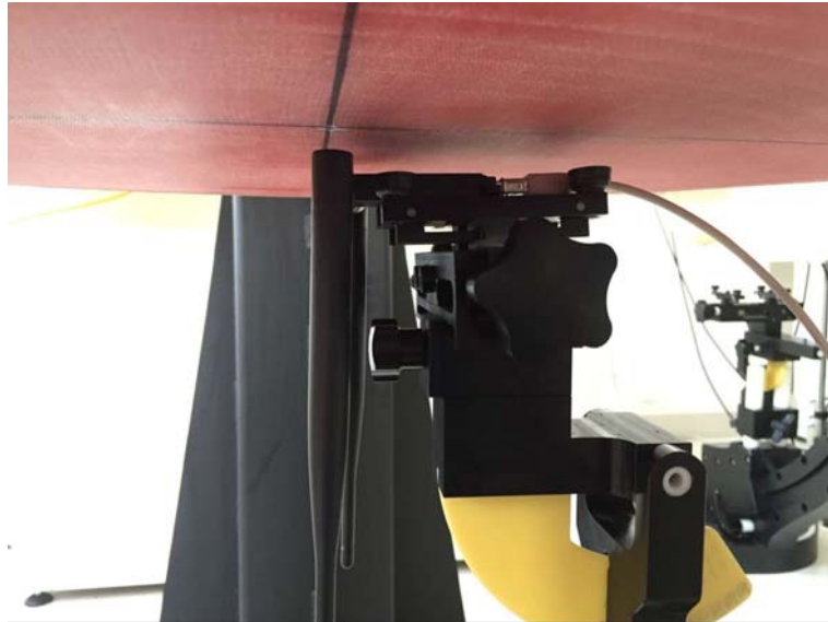
Test Position 2: 5 mm separation from the flat phantom for the bottom of the dongle at Horizontal-Down;
