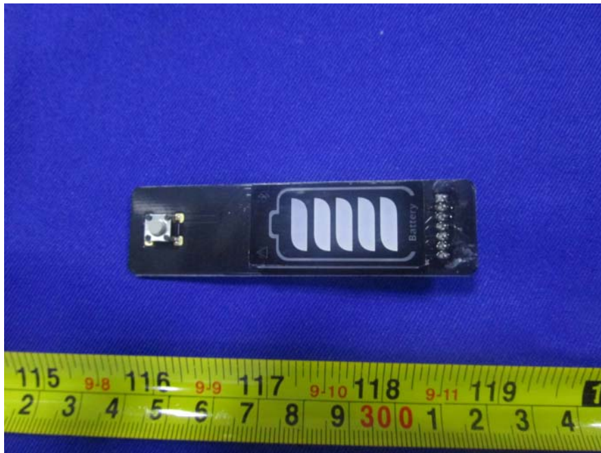
EUT – Battery Status Board Top View
