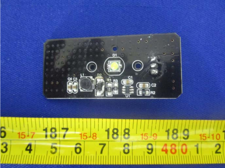
EUT – Lighting Board Bottom View
