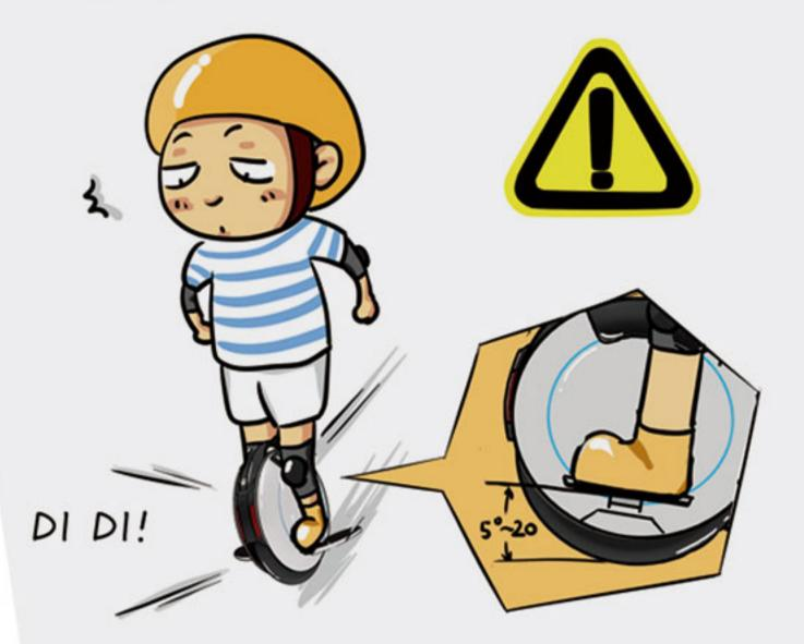
To ensure riding safety, the V5 comes with preset safe speed limit.
