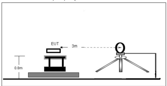
(B) Radiated Emission Test-Up Frequency 30MHz~1GHz
