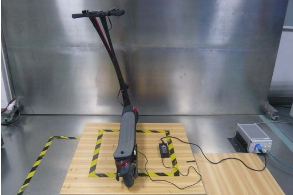
Radiated Emission View (Below 1GHz)
