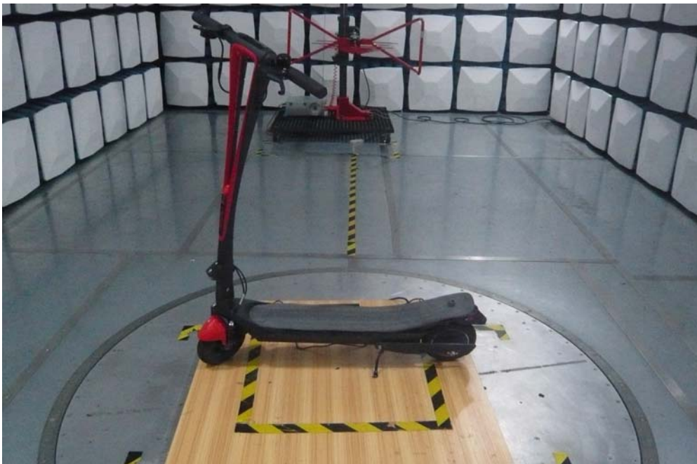
Radiated Emission View (Below 1GHz)
