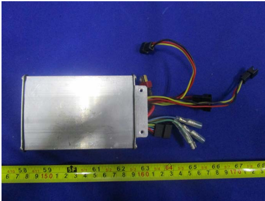
EUT – Motor Controller Bottom View
