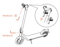
3. Place the brake lever on the handlebar, tighten it firmly with hex wrench to be sure it won't loosen. (Note: Use the M6 wrench to re-tight the folding part's nuts in case it's loosen after long time use)
