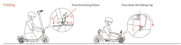
Power off the scooter, hold the stem, press the locking button and pull the lever, bend the handlebar stem towards the footrest.
