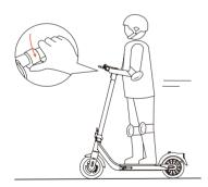
3. Stand on the footrest with both feet, press the throttle on the right hand. Note: For your safety, the motor will not engage until the scooter reaches 3 km/h.
