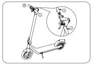
Install the handles on the stem and firmly tighten it according to the correct position and direction marked on the label
