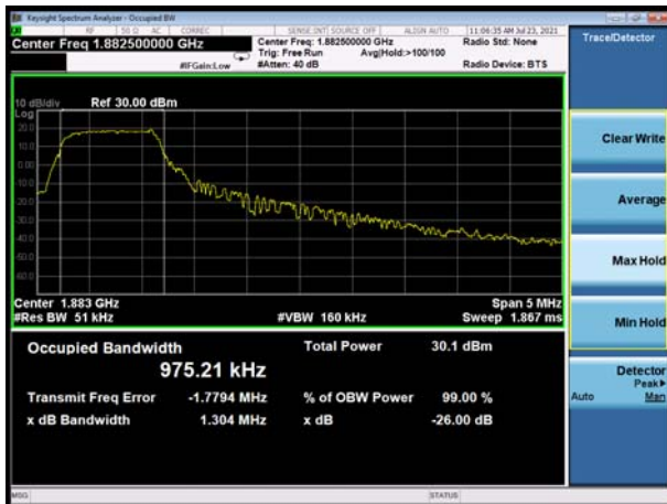
LTE eMTC Band 25 15MHz 16QAM CH-Middle
