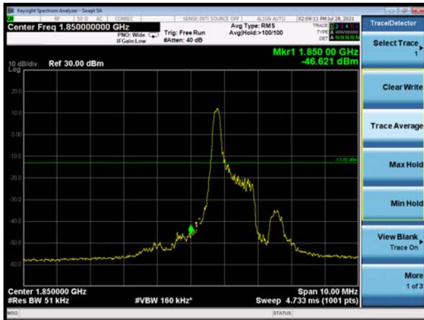
LTE eMTC Band 25 10MHz 16QAM 100%RB CH-Low
