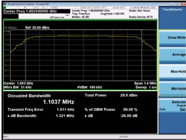
LTE eMTC Band 25 5MHz QPSK CH-Middle
