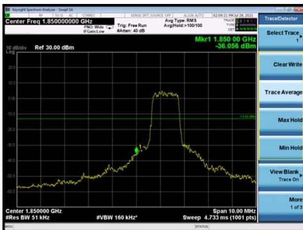
LTE eMTC Band 25 10MHz QPSK 100%RB CH-Low
