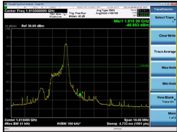
LTE eMTC Band 25 15MHz 16QAM 100%RB CH-High
