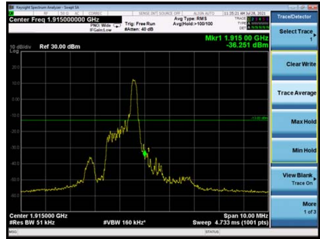
LTE eMTC Band 25 3MHz 16QAM 100%RB CH-High
