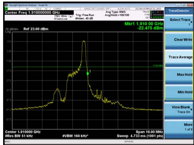
LTE eMTC Band 2 1.4MHz QPSK 100%RB CH-High
