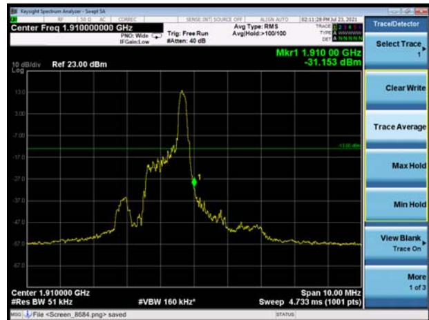
LTE eMTC Band 2 5MHz 16QAM 100%RB CH-High
