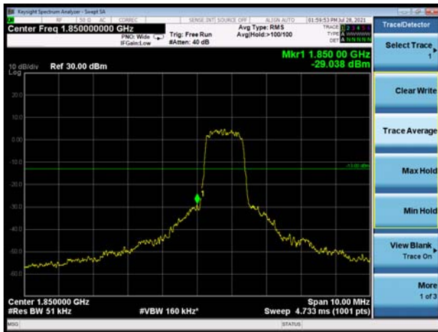
LTE eMTC Band 25 10MHz QPSK 1RB CH-Low
