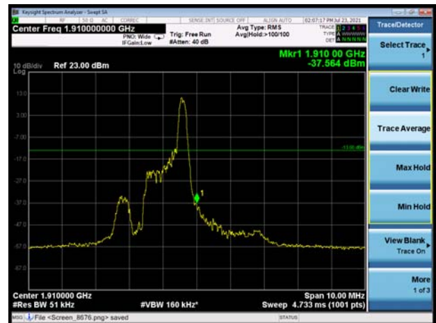
LTE eMTC Band 2 3MHz 16QAM 1RB CH-High
