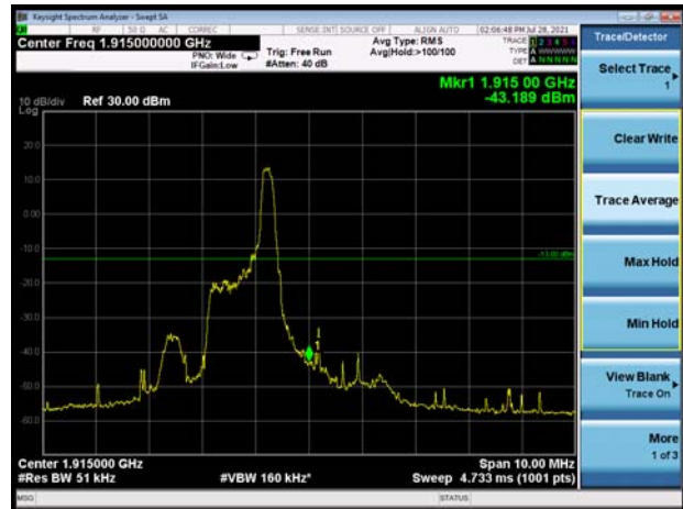
LTE eMTC Band 25 10MHz 16QAM 100%RB CH-High
