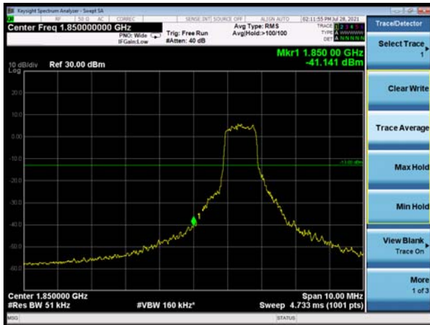
LTE eMTC Band 25 20MHz 16QAM 1RB CH-Low
