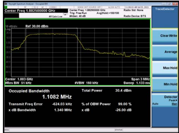
LTE eMTC Band 25 10MHz QPSK CH-Middle
