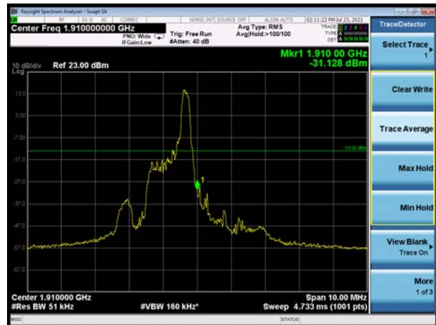
LTE eMTC Band 2 5MHz QPSK 100%RB CH-High
