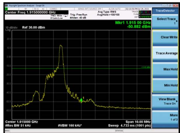
LTE eMTC Band 25 20MHz QPSK 1RB CH-High
