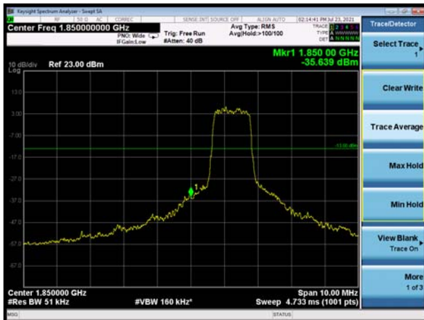
LTE eMTC Band 2 15MHz QPSK 1RB CH-Low
