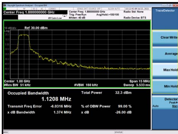
LTE eMTC Band 2 15MHz QPSK CH-Middle
