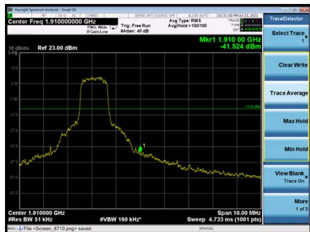
LTE eMTC Band 2 20MHz QPSK 100%RB CH-High
