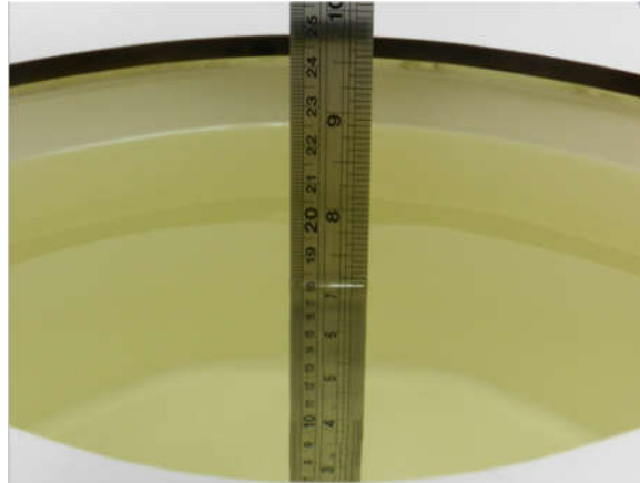
Fig 10.1 Photo of Liquid Height for Body SAR
