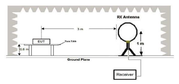
(2) Radiated Emission Test-Up Frequency 30MHz~1GHz
