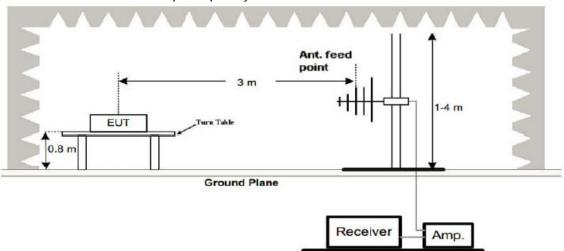
(3) Radiated Emission Test-Up Frequency Above 1GHz
