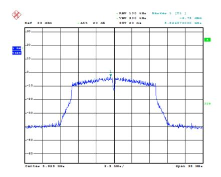
*Chain 2 Test Mode: 802.11n-HT20* 5745MHz
