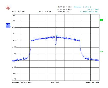
*Chain 1 Test Mode: 802.11ac-HT80* 5775MHz
