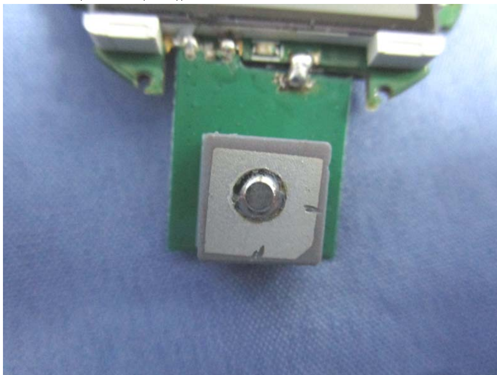
(19) EUT Photo (Antenna (GPS))
