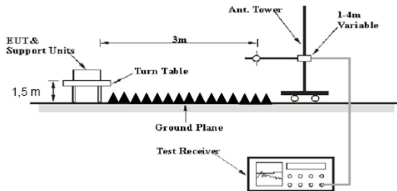
The radiated emission tests were performed in the 3 meters test site, using the setup accordance with the ANSI C63.10-2013. The specification used was the FCC 15.209, and FCC 15.247 limits.
