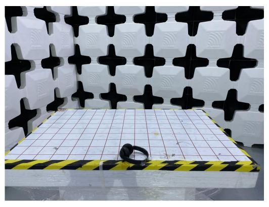
(The EUT placed at the center of turntable)
