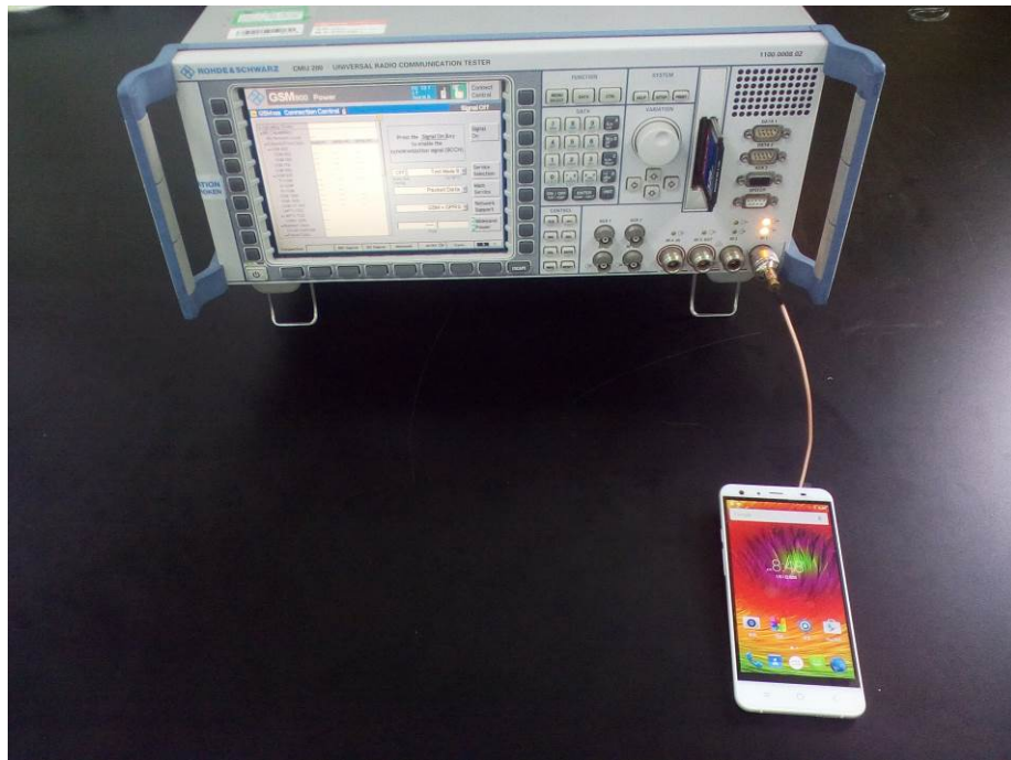
Photograph –2G&3G Conducted Test Setup
