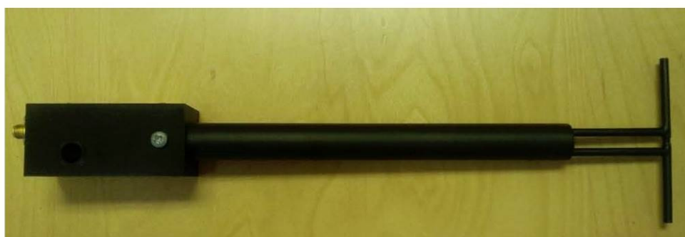
Figure 1 – MVG COMOSAR Validation Dipole
