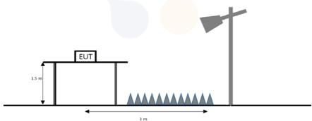
The diagram below shows the test setup that is utilized to make the measurements for emission from Above 40 (#z emissions.
