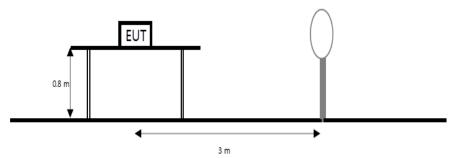
The diagram below shows the test setup that is utilized to make the measurements for emission from 30 Mz to 1  $\mathbb{G}$  emissions.
