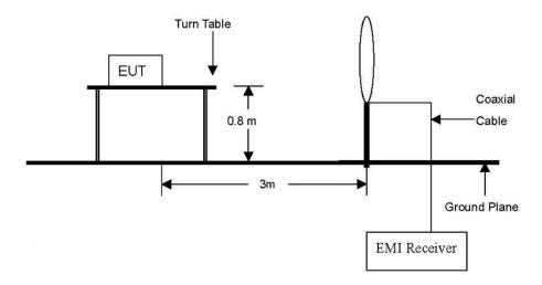
The diagram below shows the test setup that is utilized to make the measurements for emission from 30 Mz to 1 Gz emissions.
