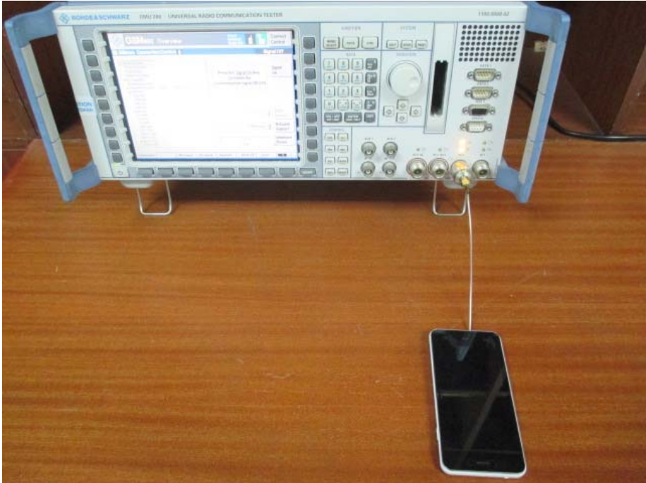
Photograph – 2G&3G Conducted Test Setup
