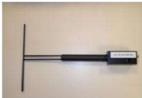
Figure 1 – Satimo COMOSAR Validation Dipole
