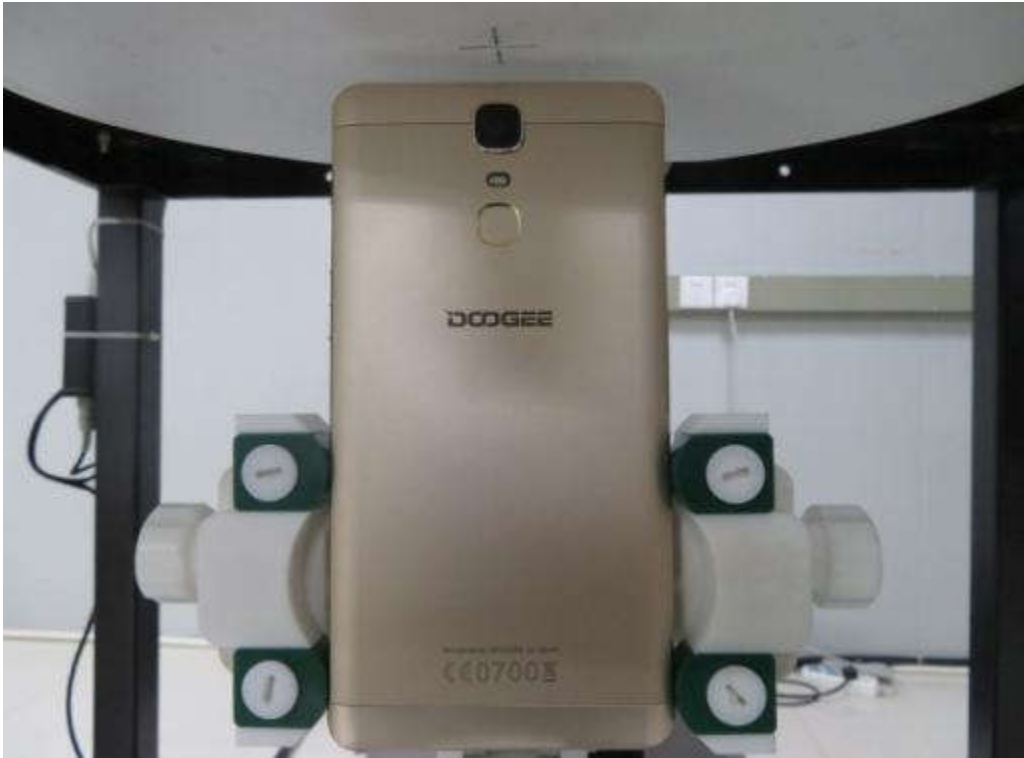
10mm body-worn Top Side Setup Photo(hotspot)
