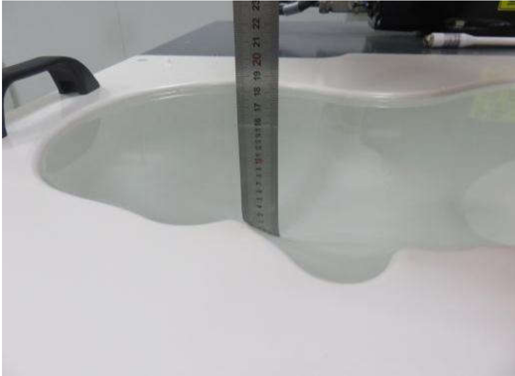
Photograph of the depth in the Head Phantom (750MHz, 15.9cm depth)
