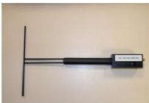
Figure 1 – Satimo COMOSAR Validation Dipole
