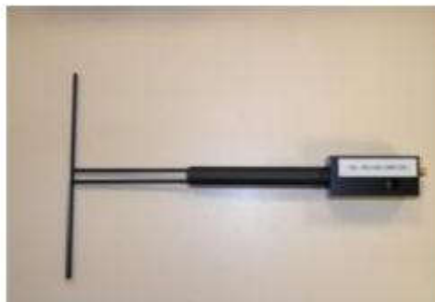
Figure 1 – Satimo COMOSAR Validation Dipole
