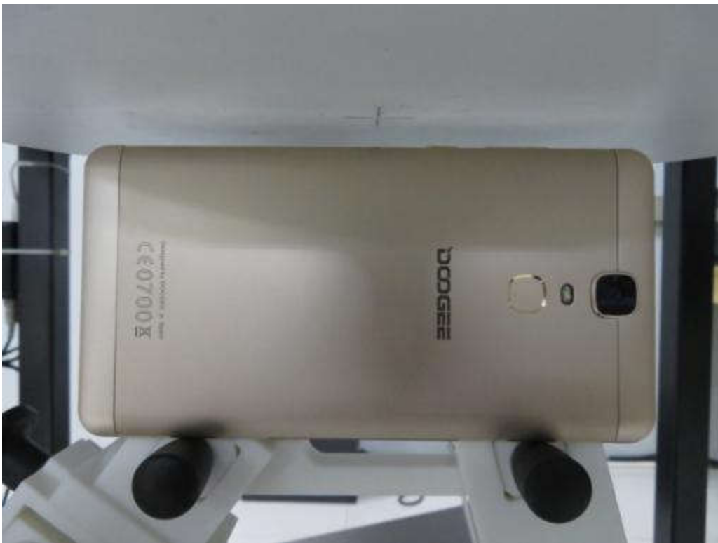
10mm body-worn Right Side Setup Photo(hotspot)
