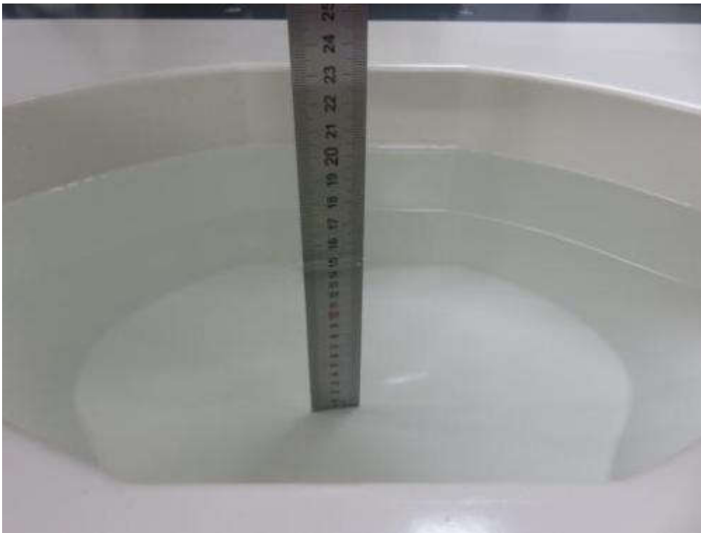
Photograph of the depth in the Body Phantom (2600MHz, 16.2cm depth)
