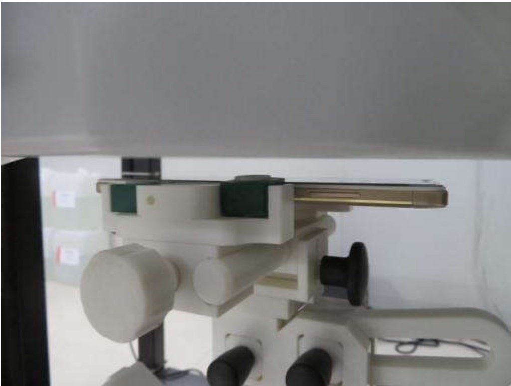
10mm body-worn Front Side Setup Photo
