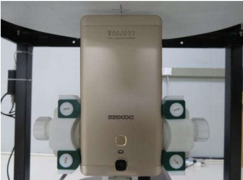
10mm body-worn Bottom Side Setup Photo(hotspot)
