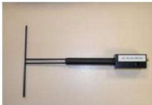
Figure 1 – Satimo COMOSAR Validation Dipole
