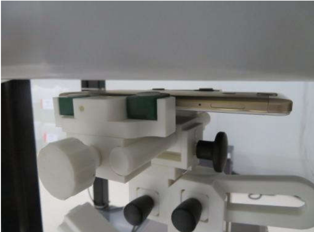
10mm body-worn Back Side Setup Photo
