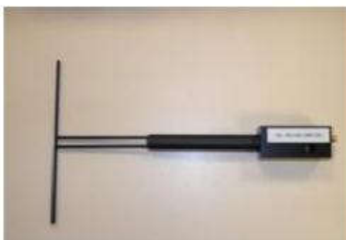
Figure 1 – Satimo COMOSAR Validation Dipole
