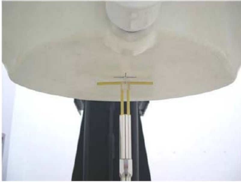
Fig 7.2 Setup Photo of Dipole Antenna
