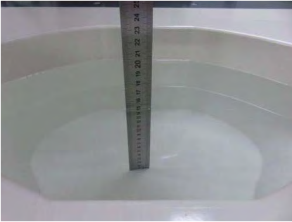
Photograph of the depth in the Body Phantom (2450MHz, 15.7cm depth)
