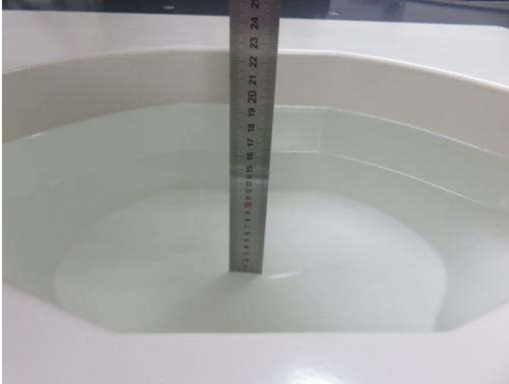
Photograph of the depth in the Body Phantom (1900MHz, 16.2cm depth)
