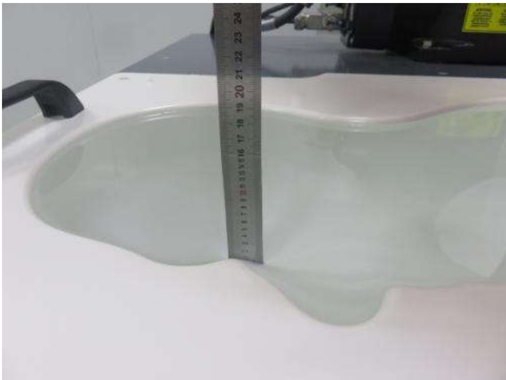
Photograph of the depth in the Head Phantom (1900MHz, 15.6cm depth)
